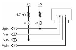
For 1-Wire I/O using a Blue Dot Receptor, configure the RJ-11 port as follows (J3 in):
