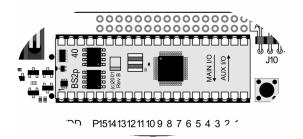
The BS2p40 module can be programmed via the USB port or through a standard serial port.
