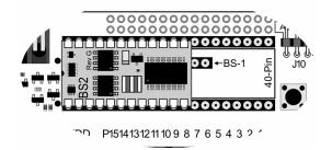
The 24-pin BASIC Stamp or Javelin Stamp module can be programmed via the USB port or through a standard serial port. A 24-pin BASIC Stamp and Javelin Stamp modules may be used in conjunction with an installed SX28AC/DP micro.
