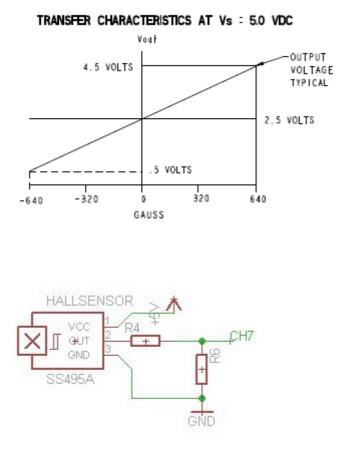
This output voltage is digitize to a 12bit digital value and this value is read by the microcontroller software.
