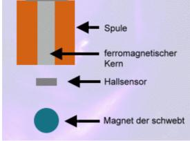
Spule ... solenoid ferromagnetic core hallsensor floating magnetic object
