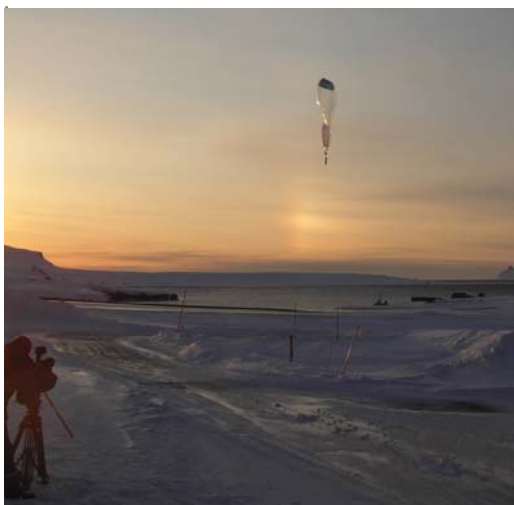
Figure 2. CMET balloon launched from Ny-Ålesund Svalbard, Norway. The balloon was shipped in a small package and operated from the United States. Photo Credit: Lars Hole
