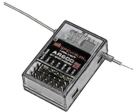
Figure 6. Typical RC Receiver (6-channel Spektrum AR600 is shown).
