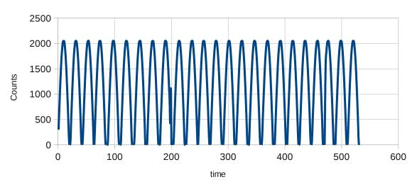
Capture of 100HZ sine wave from the working channel of the digitizer. (Yeah, HP3312A, ebay special, great price, needs cal/adjust) Output from BST terminal log-captured and graphed using Libre Office spreadsheet.
