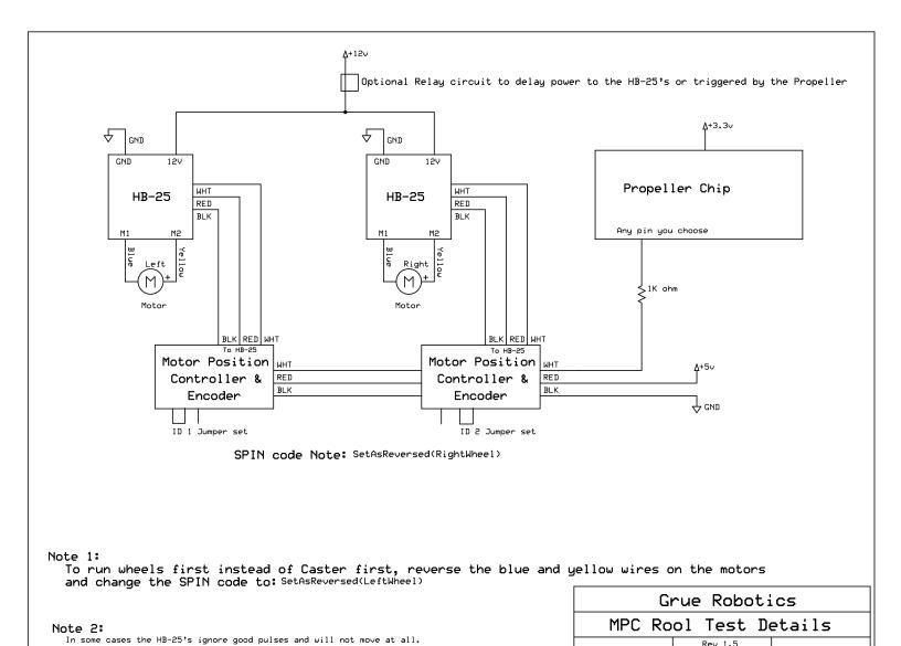
The work around to this is to delay power to the HB-25's until after the Propeller powers up
