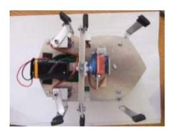
View from below – NB - no battery holder in this pic – just used tape – leaving the battery in usual position on BOE disturbs balance of the walker
