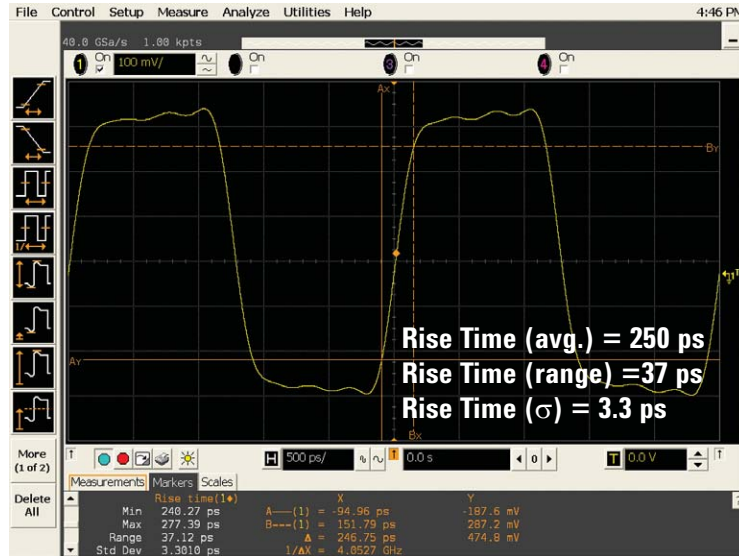
Figure 15a: 400-MHz clock captured on an Agilent Infiniium DS080304A 3-GHz oscilloscope sampling at 40 GSa/s
