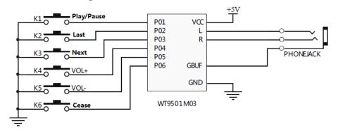
L, R GND connect to external amplifier (GBUF is not recommended):
