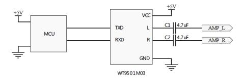
L, R GND connect to external amplifier (GBUF is not recommended):
