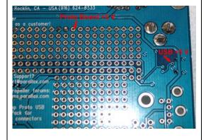
2/ Solder a 2-way header to the Protoboard +5 V hole.
