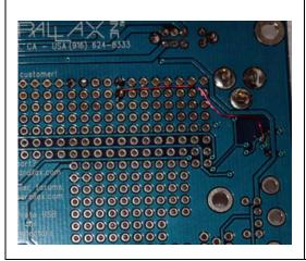
4/ Fit a jumper to connect USB +5 V to Protoboard +5 V
