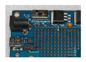
3/ Carefully scrape the solder resist from the USB +5 V via and solder a fine wire link between the USB +5 V via and the bottom pin of the header.
