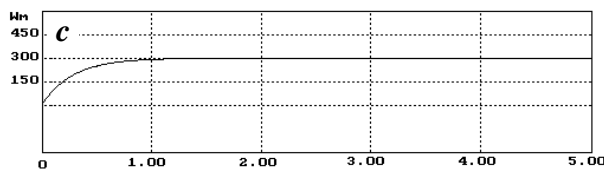
Figure 8. Starting characteristics by (a) PI controller, (b) PID controller and (c) PID control by neural network.
