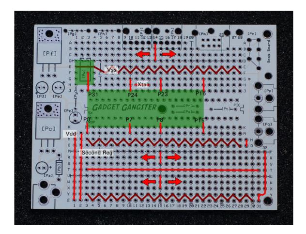
Setting up the Boss Board for the Propeller: [Pc] - 3.3v regulator - P1= Ground, P2 = Vout, P3 =Vin [Pf] - Secondary regulator - P1=Ground, P2 = Vout, P3=Vin. Only powers M1 - Z1
