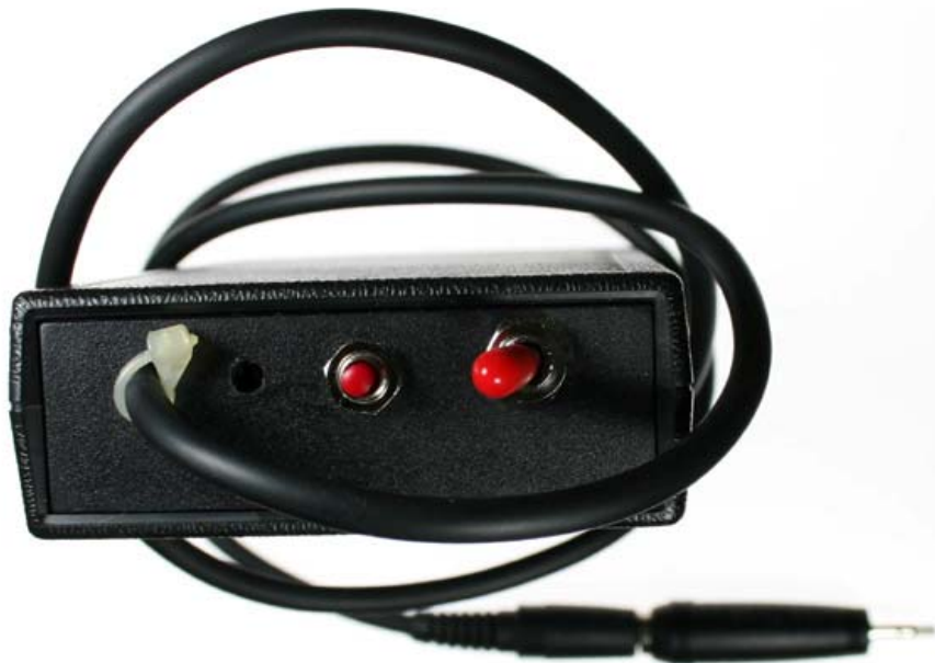
Figure 8. Front view of the CamTimer showing the switches.
