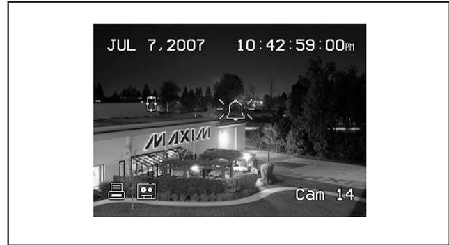
Figure 1. CVBSOUT with the First OSD Display in Demo Mode (NTSC)
