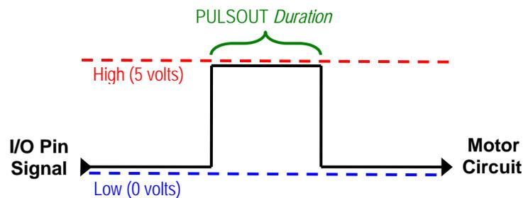
The Scribbler wheels' motor circuitry is waiting for a high (5 volt) signal pulse, and when it gets one, it will measure how long it lasted.
