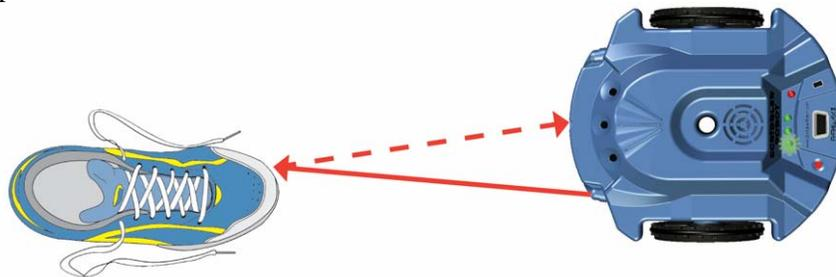
Infrared light reflects easily off of shiny, light-colored surfaces, but it is absorbed by dull, dark-colored surfaces. So, the infrared object detection system will be able to see a white rubber sneaker better than a black velvet slipper.
