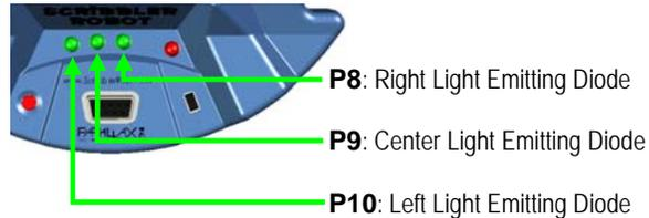
makes an I/O pin connect an LED circuit to 5 volts, which turns on that LED. Even though the BASIC Stamp executes the commands one at a time, it looks like the LEDs all turn on at the same moment. That is because computers work faster than our eyes can see. Sometimes we need to slow them down to human speeds. The next command does just that:
