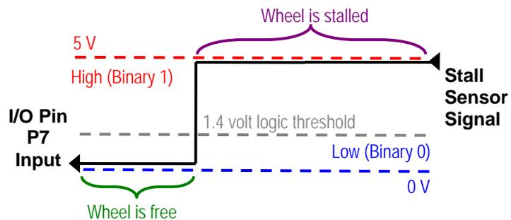
To receive the signal from the stall sensor, I/O pin P7 needs to be set as an input. You can use the `INPUT` command to do this, but it is often not necessary. Input is the **default mode** for BASIC Stamp I/O pins: they are automatically set to input unless you put a command in a program that uses them as an output.
