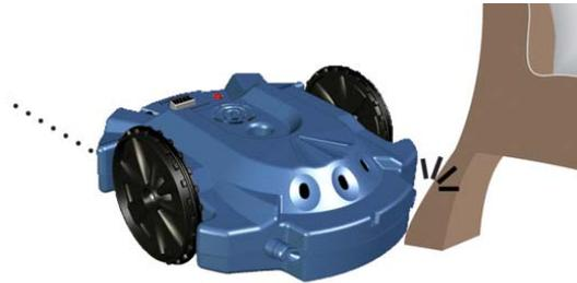
When the motors are running and the wheels can turn freely, the stall sensor sends a low voltage signal to I/O pin P7. If the motors are running but either one of wheels can't turn, the stall sensor sends a high signal to P7.
