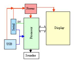
The device consist of an interface, USB interface, power supply, processor and sounder as shown in the block diagram.
