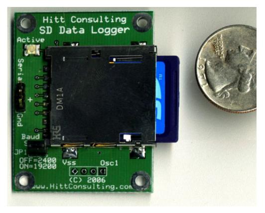
The SD Data Logger allows any microcontroller that can send and receive serial data to create files on SD
