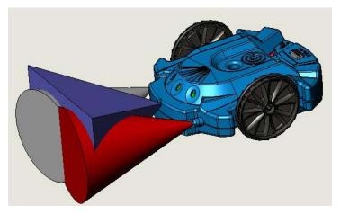
The two IR LEDs on the front of the Scribbler emit modulated infrared light. The IR detector between them is tuned to see this light reflected off of objects.
