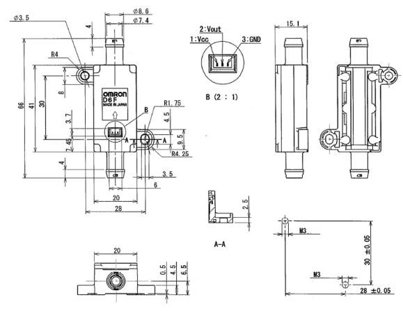
Note: Mount using an M3 pan head screw, tightened to 0.59 N•m max. torque.
