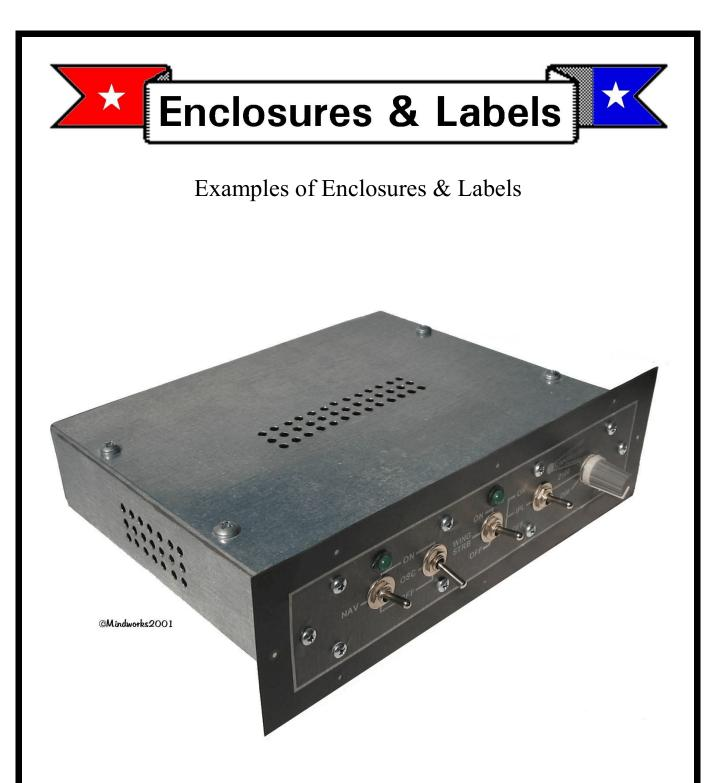
Picture NSI 1....This Enclosure, Label and Electronics was designed for an Experimental Aircraft which controls the Navigation, Strobe and Instrument panel Lights....This Panel mounted Enclosure is approximately 7-3/8" W x 6" D x 1-1/2" H ....
