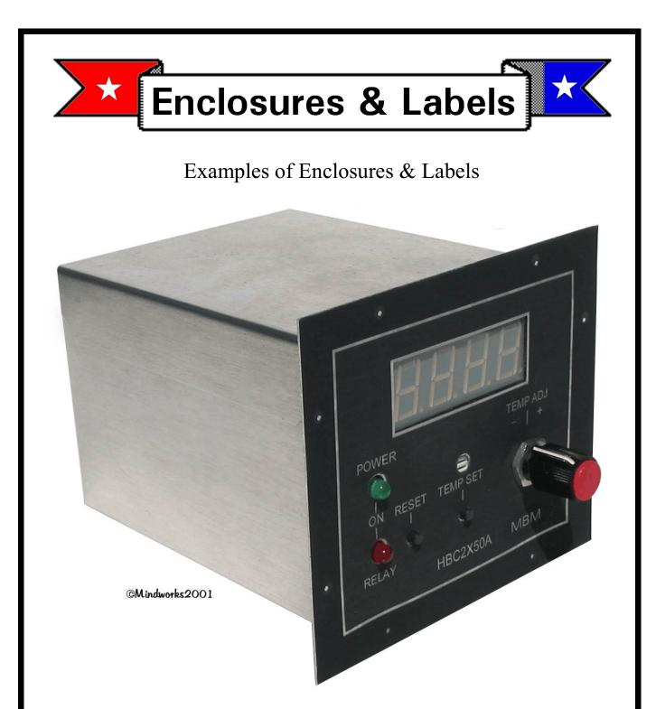
Picture NSI 6....Here is a picture of NSI 5 with the components and label installed. This unit was designed to control and regulate the Temperature of a Molded injection cylinder through the use of two SSR's rated at 110-220 Vac @ 50 amps each. Each SSR is coupled to a heater band. Temperature monitoring and control are by means of a Thermocouple unit and is adjustable from 32F -600F. All Microprocessor controlled. The Enclosure is Panel mounted.
