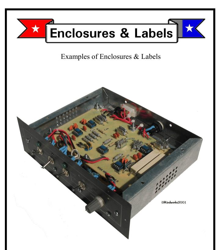
Picture NSI 2....Here is an internal view of the NSI 1 showing the two custom made PCB's. One on top of the other. Very Compact....
