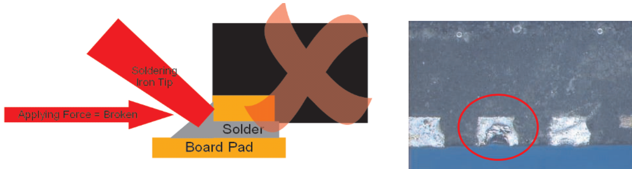
Figure 18. Manual Rework Damage
