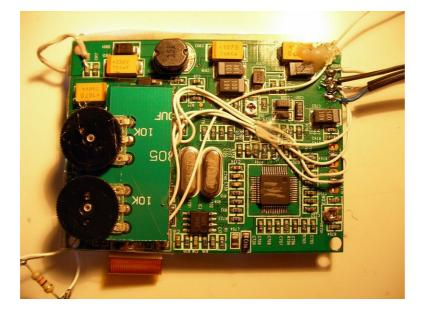
I hot glued this board onto the back of the LCD board with a sheet of plastic between for insulation.
