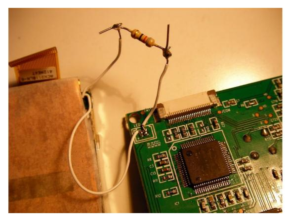
The resistor in series with the LEDs. This should be done more neatly and insulated and you don't have to change the wires from the originals (long story).
