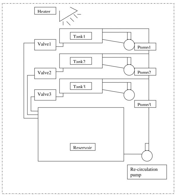
Heater: 208VAC,10.5 amps. Turned on by 24 VDC relay. 24 VDC relay turned on by 5VDC (BS2).
