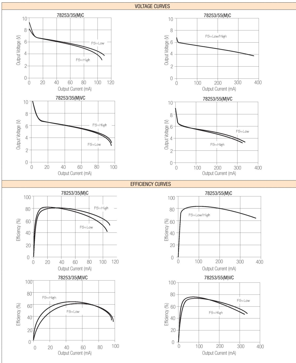
All curves are derived from testing with the Maxim MAX253 IC using the circuit shown in application note MPAN-03 ( download at <http://www.cd4power.com/data/apnotes/mpan-03.pdf>).
