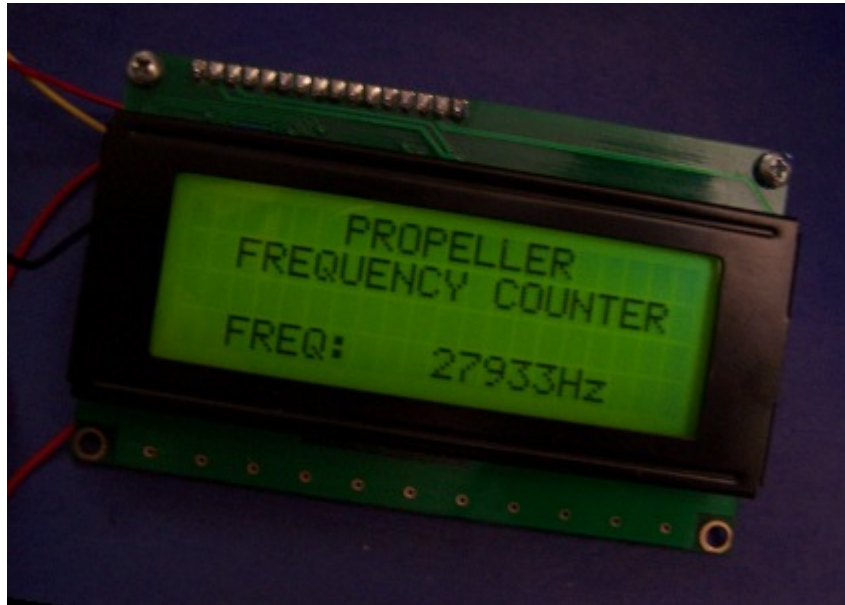
(This frequency reading is exactly the same reading using an HP 5314A)
