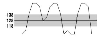
Notice, however, that for maximum accuracy, we need to keep track of where the waveform crosses the centerline – *not where it exits the hystersis band* – to locate the edges of the bars. The hysteresis band exists simply to determine whether a given centerline crossing is real or not.
