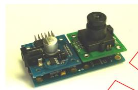
MoBoStamp-pe, assembled with PWR-I/O-DB and TSL1401-DB
