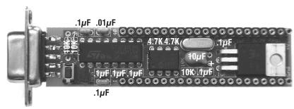
of the board. (That way, the socket strip will keep it from sliding out.) Solder the crystal into place.
