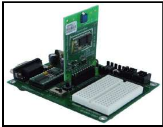
Figure 2: The Board Of Education carrier board with the EB500 connected.
