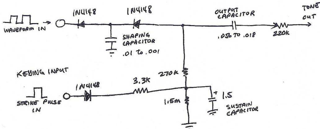
A couple of afterthoughts: If some of the waveform bleeds through during a non-keyed period, it may help to slightly raise the baseline of the oscillator signal above ground level. This can be done either by running it through an op amp ahead of the keying diodes with a slight offset voltage on the + input, or by creating a resistor network with a voltage divider and ballast resistor ahead of the keying diodes, pulling up the baseline.
