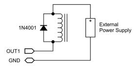
Note the addition of the 1N4001 suppression diode when using the external supply. This is recommended because the diodes internal to the ULN2803 are not connected to the external supply when using this configuration.
