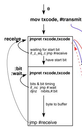
0) The full duplex serial pasm cog is started, and it goes through an initialization procedure which concludes with the **mov** instruction shown at the top of the diagram. The impret mechanism depends on two cog registers, rxcode and txcode that will be used to store addresses for indirect jumps.
