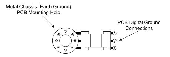
Detail of Floating Mounting Hole with Option for Digital Ground Connection
