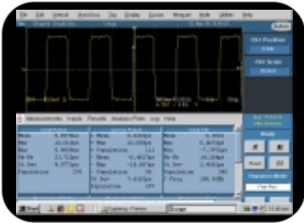
▶ Figure 56. The TDSJIT2 optional software package for the TDS7000 Series oscilloscope is specifically designed to meet jitter measurement needs of today's high-speed digital designers.
