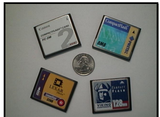
Photo 1—CompactFlash cards are available from a variety of manufacturers in several different capacities.
