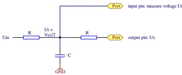
Ut charge/discharge when  $U_{in}$  is constant and  $C$  charged
