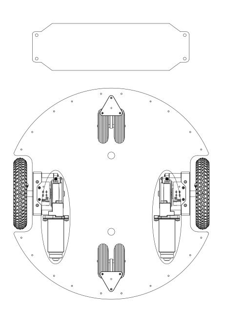
1/2" Maple Plywood Robot Base for Caster Wheel (#28971) and 12V MMWK (#27971)
