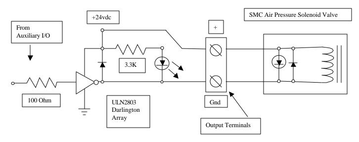
Note: The red LED's, light up to indicate a load at this output is energized.
