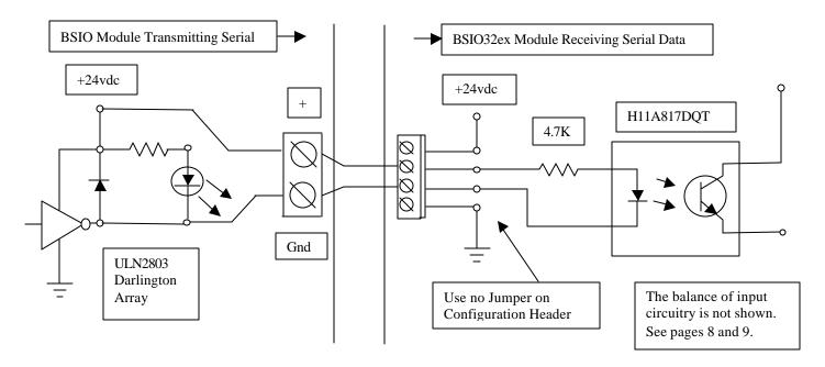
A logical "1" placed on the output driver of the transmitting module will translate to a logical "1" on the input pin of the receiving module. A BSIO16 module may also transmit serial data to a BSIO32ex module using this wiring configuration. Note: This mode of serial communication is not bi-directional.
