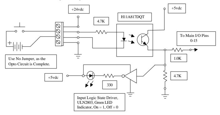
The opto-isolator can be used to import a digital signal from another powered device, while maintaining electrical isolation. Note: Use only DC sources; AC signals will damage the LED in the opto-isolator. To input an AC signal source, run the AC signal power through a full wave rectifier with an output filter capacitor and maintain correct polarity when connecting to the input terminals. The filtered output should not exceed 24 - 30 volts DC.
