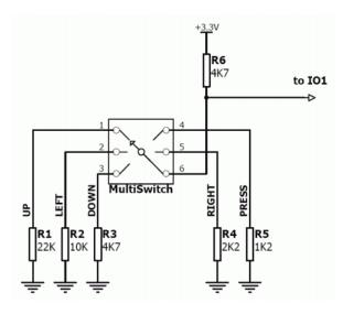
Unused buttons do not need resistors to be connected to the circuit. Table below lists the buttons and corresponding resistor values.
