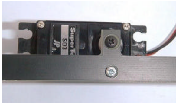
Leg assembly fitted to the horn and loosely fitted to the servo
