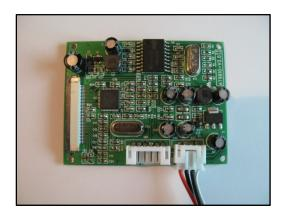
We recommend that VCC be 5V DC, but we have seen the driver board operate from 3.8V DC to 7.0V DC. When the voltage approaches the lower end range the image may become blurry fuzzy and the image may not hold still. We only tested up to 7.0V DC, but suspect the display may operate well at a higher voltage. When operating at 5V DC, the display and drive PCB require approximately 150mA.
