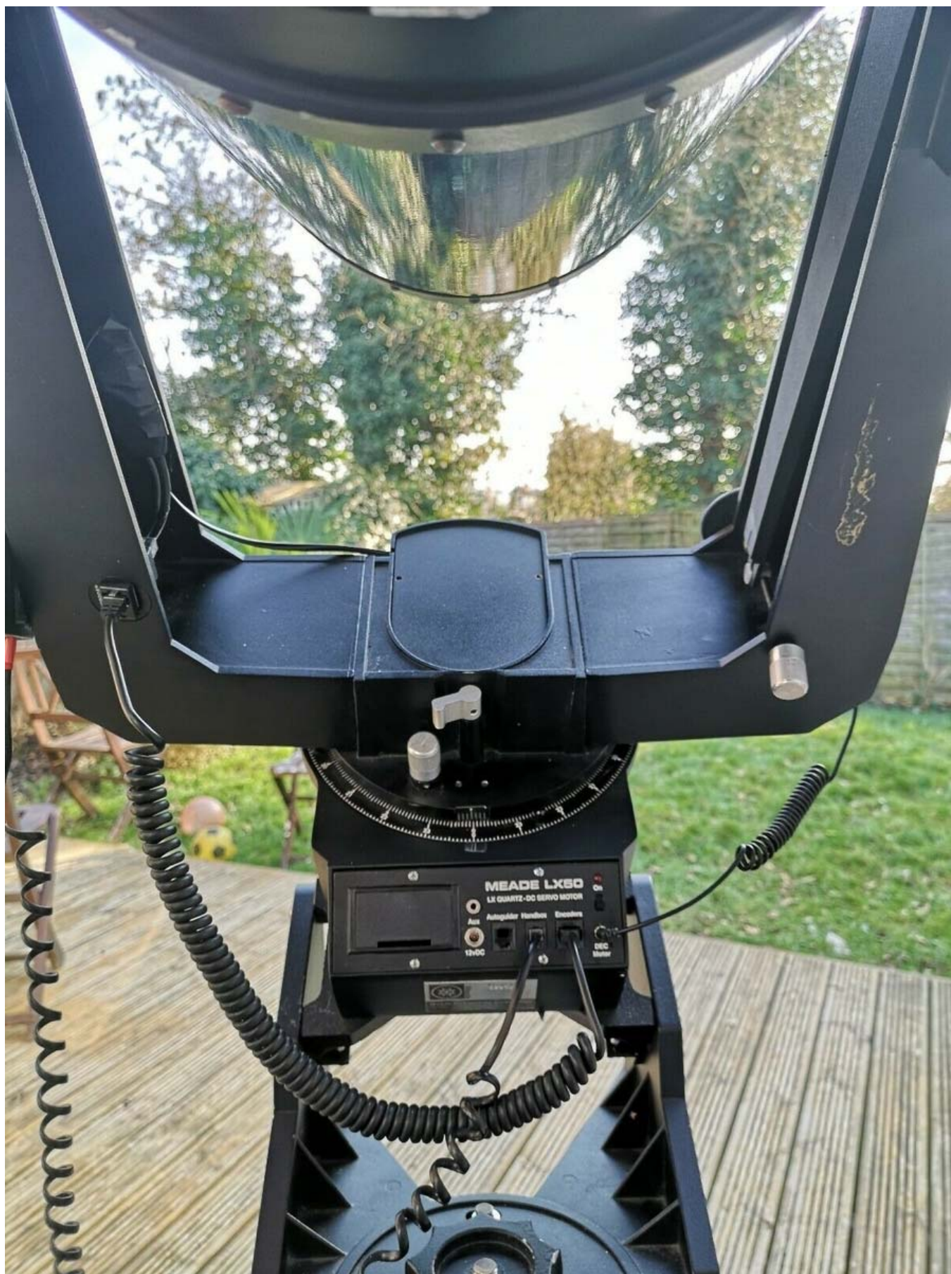
LX50 Telescope with Control Panel. Encoders and Handbox connected.
