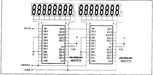
Figure 3. Cascading MAX7219s to drive 16 7-segment LED digits.
