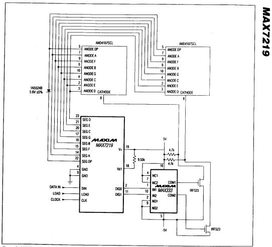
Figure 2. MAX7219 Driving 4 Inch Displays
