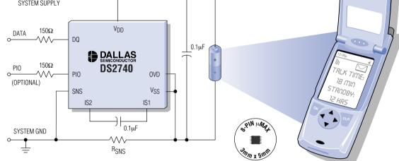
The DS2740's 15-bit current measurement has a resolution of 78 $\mu$ A and a 2.56A dynamic range when used with a 20m $\Omega$  sense resistor. An analog input filter extends this dynamic range for pulse-load applications. With a current ADC offset of less than 2 $\mu$ V and a gain error of less than 1%, the DS2740 provides a highly accurate report of remaining battery capacity.
