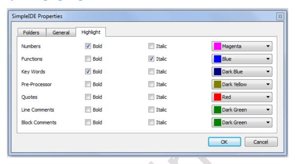
The Highlight properties tab can be used to change editor syntax colors. At this time only a select set of system colors is available.
