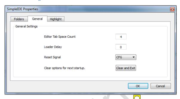
Some general property details may need to be changed for different boards. For example, some USB serial devices do not have DTR for controlling Propeller reset and should use RTS instead. You can change the Reset Signal from DTR to RTS if necessary. in the properties "General" tab. This can be changed at any time.
