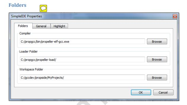
In most cases, the Folders tab will already have the fields properly set. The back-slash '\' folder separators used in windows are replace by '/' in the IDE. Please take note of the fields and click OK when ready. The Compiler and Loader Folder must be set correctly pre you can move to the next step. You should choose a work-space if one is not already set. You can skip to Paring the Helio Demo when the folders are properly set.
