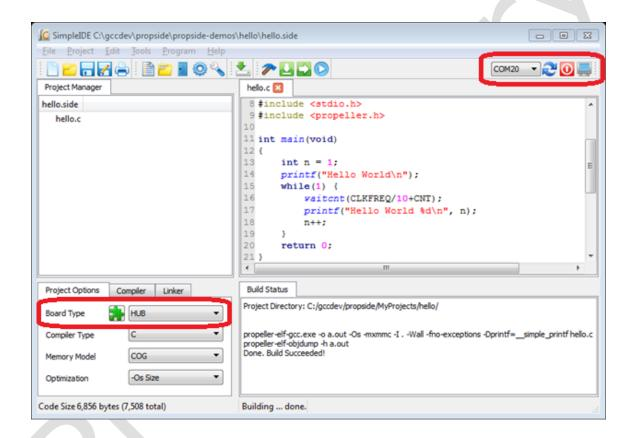
The Hello demo should be run with a simple board type like HUB like shown above.
