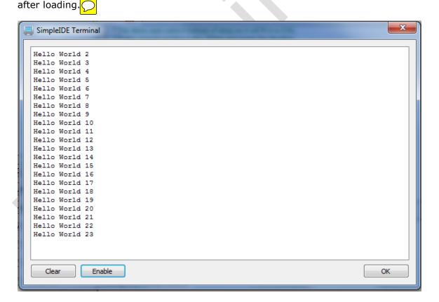
Note that the terminal is not fast enough to catch the first few hello lines. This is because of the transition from propeller-load loading the program, releasing the serial port, and starting the terminal.
