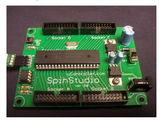
The SpinStudio Mainboard is the base to which the peripheral boards are attached. It consists of...
