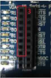
We are going to place our jumper wires into the headers on both the VGA header strip and the I/O pin header strip.
