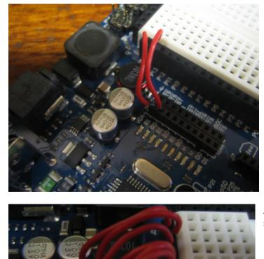
Then insert a jumper wire into the next pins down. Keep doing this until you get to pin P8.
