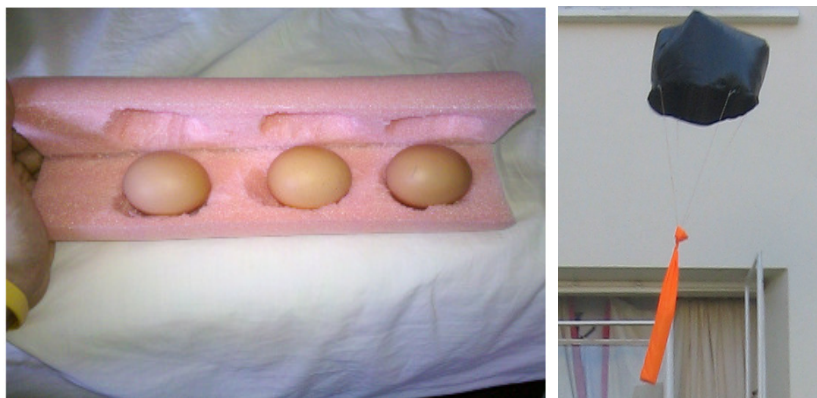
Figure 23 The eggs in a section of Pool Noodle and the parachute in action during the Parachute Test
