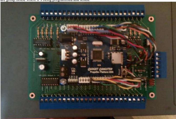
The Spinneret will be connected at SIO2, which is just to the right of the SD card slot on the Propeller Platform. The inputs where the Bilge floats will be connected too are on the top and the outputs are where Alarm Horn/Light relay and F/A Horn Silence relay are connected on the bottom right. The 12VDC power supply that is located on the left of the Propeller Platform will be able to supply 1 amp of power for the Spinneret and the Propeller Platform from the +VOUT on the I/O board.
