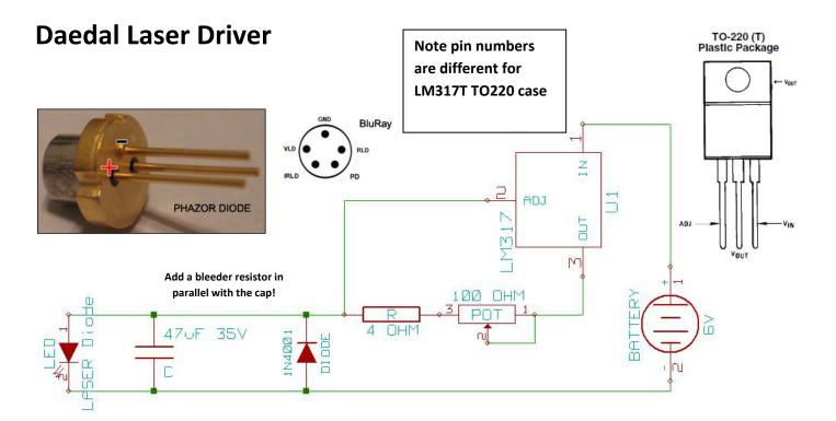
The LM317 uses 1.25 volts for its reference voltage:
